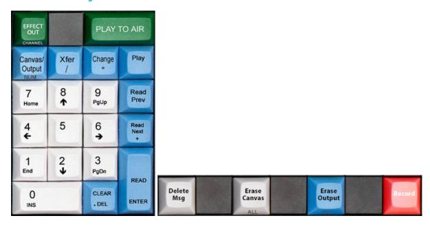
The Classic keyboard uses multi-colored keys so operators can have quicker access to critical sections of the keyboard.
