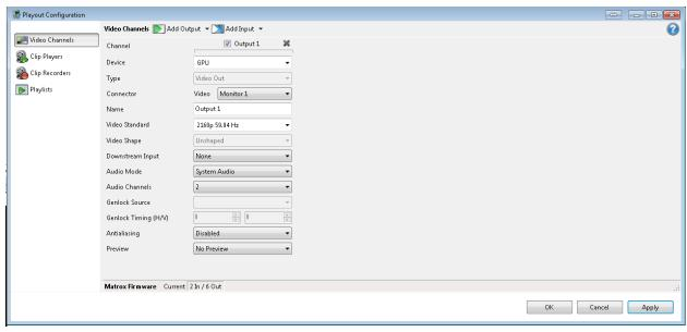
Please note the Video Standard resolution is nonstandard. With this Setup, it allows us to configure 1 GPU across 4 Monitors Maximum
