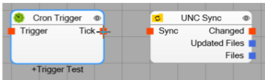
Lesson STYLEREF \s "Überschrift 1" 2. SEQ Lesson \* ARABIC \s 1 9 – Connecting Cron Trigger and UNC Sync nodes
