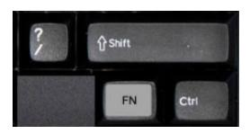
When the "FN" modifier key is pressed a secondary function on certain keys will be sent. These secondary functions are indicated by legends on the front of the key The secondary function is activated if the button is pressed while the FN key is held down. The FN key is located just to the right of the space bar and is light grey for easy identification.
