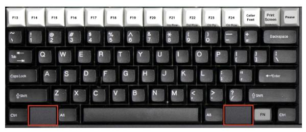
The operating system keys such as the "Win" and "App" keys have been removed from the critical typing areas to prevent accidental use during live productions. These OS functions can always be accessed by on screen methods with the mouse. Additionally, the "Win" key was moved to the top left of the keyboard.
