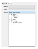
Clicking on the Stopped drop down box a list of items that can be triggered is presented. Check the Timer1\_Stopped item under Scripting and the **Timer1\_Stopped()** method will be automatically added to your scene script.
