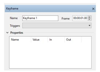
The drop down will display all the events that the keyframe can trigger. We are interested in the Scripting option were **KeyFrame1\_Trigger** can be checked or unchecked.
