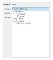
Clicking on the Finished drop down box a list of items that can be triggered is presented. Check the Timer1\_Finished item under Scripting and the **Timer1\_Finished()** method will be automatically added to your scene script.
