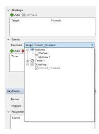
Clicking on the Finished drop down box a list of items that can be triggered is presented. Check the Timer1\_Finished item under **Scripting** and the **Timer1\_Finished()** method will be automatically added to your scene script.
