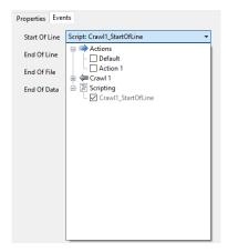
Check the Crawl1\_StartOfLine item under **Scripting** and the **Crawl1\_StartOfLine()** method will be automatically added to your scene script.
