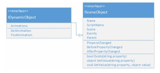
The **IDynamicObject** is the base interface for graphics and effects scene objects. It extends the functionality of the **ISceneObject** described earlier.
