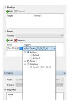
Clicking the Add button in the Timer Events property section will add an event that can be triggered based on the time set in the *Timer* column. Click the Triggers next to the Time and a list of available items that can be triggered will be displayed. Checking the Timer1\_00\_01\_00\_00 will add the **Timer1\_00\_01\_00\_00()** method automatically to the scenes script.
