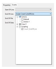
Check the Crawl1\_EndOfLine item under **Scripting** and the **Crawl1\_EndOfLine()** method will be automatically added to your scene script.
