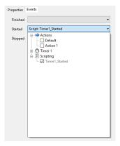
Clicking on the Started drop down box a list of items that can be triggered is presented. Check the Timer1\_Started item under Scripting and the **Timer1\_Started()** method will be automatically added to your scene script.
