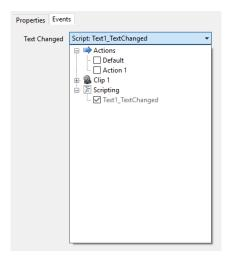
Check the Text1\_TextChanged item under **Scripting** and the **Text1\_TextChanged()** method will be automatically added to your scene script.
