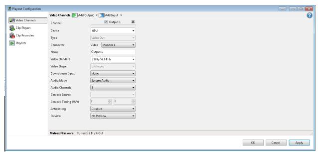
Please note the Video Standard resolution is nonstandard. With this Setup, it allows us to configure 1 GPU across 4 Monitors Maximum
