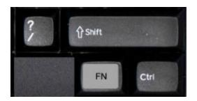
When the "FN" modifier key is pressed a secondary function on certain keys will be sent. These secondary functions are indicated by legends on the front of the key The secondary function is activated if the button is pressed while the FN key is held down. The FN key is located just to the right of the space bar and is light grey for easy identification.
