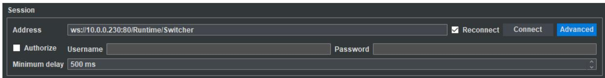
The screenshot shows the 'Session' configuration window with the 'Advanced' tab selected. The 'Address' field is still 'ws://10.0.0.230:80/Runtime/Switcher'. The 'Reconnect' checkbox is checked. The 'Connect' button is disabled, and the 'Advanced' button is highlighted in blue. Below the address field, there is a checkbox for 'Authorize' which is unchecked. To the right of the 'Authorize' checkbox are two text input fields: 'Username' and 'Password'. The 'Minimum delay' field is still '500 ms'.
