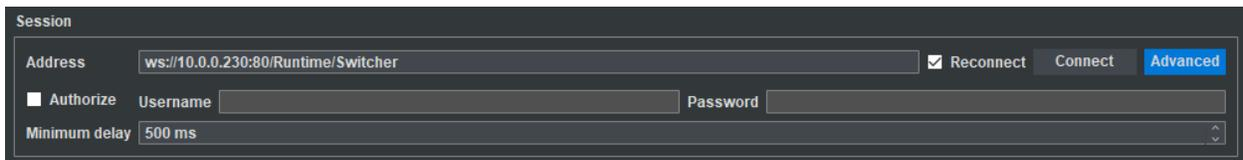
The screenshot shows the 'Session' configuration window with the 'Advanced' button highlighted in blue. The 'Address' field is 'ws://10.0.0.230:80/Runtime/Switcher', 'Reconnect' is checked, and 'Minimum delay' is '500 ms'. There are 'Authorize', 'Username', and 'Password' fields.
