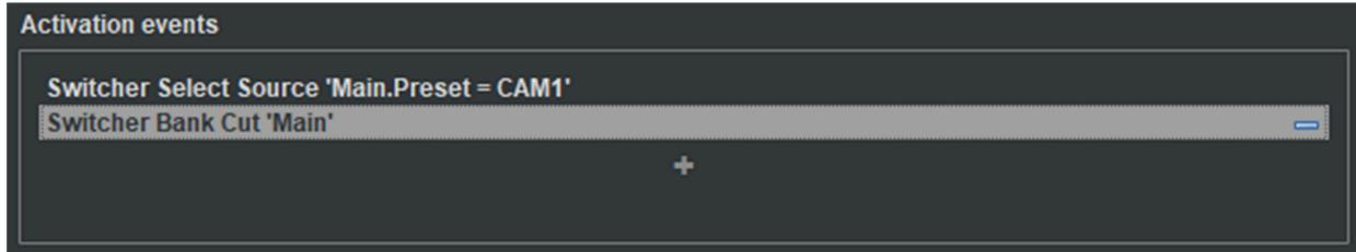
**NOTE:** When planning Activation and Deactivation Events, it is best practice to program the transitions in either the Activation Events or the Deactivation Events - not in both; otherwise, a double transition will be performed. For example:
