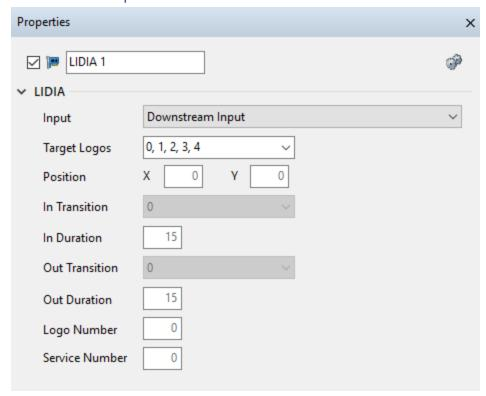
Input: Select the input video source containing VANC triggers
