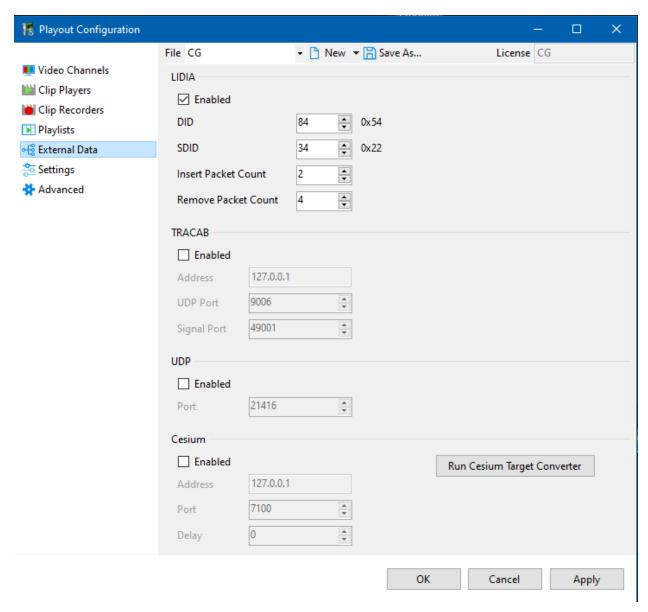
The LIDIA decoders detect a trigger signal on line 9 of the HD SDI <u>V</u>ertical <u>ANC</u>illary (VANC) data space.
