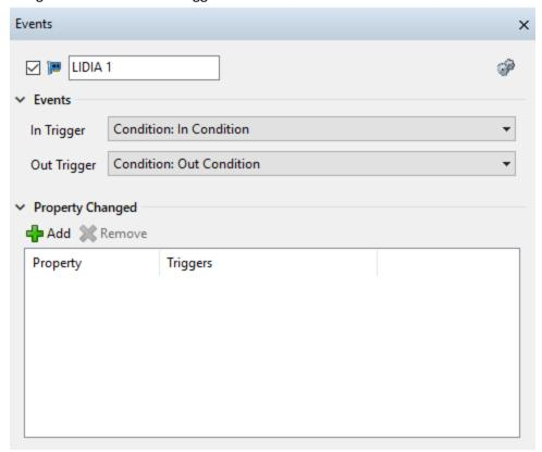
In the above example we define the "In" & "Out" Triggers to be triggered by the VANC triggers. In this example we will execute PRIME "Conditions" "Condition In" and "Condition Out" to evaluate what PRIME transition to execute upon receiving the VANC triggers.
