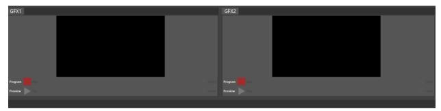
PRIME Switcher comes with two channels of graphics internally. Graphics can be controlled a few different ways:
