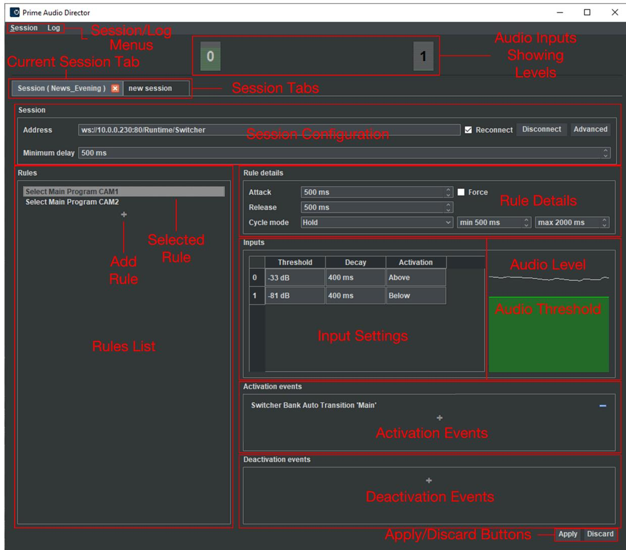
**NOTE:** If an Audio Input Level does not display, then ensure that the audio source is connected and operating properly.
