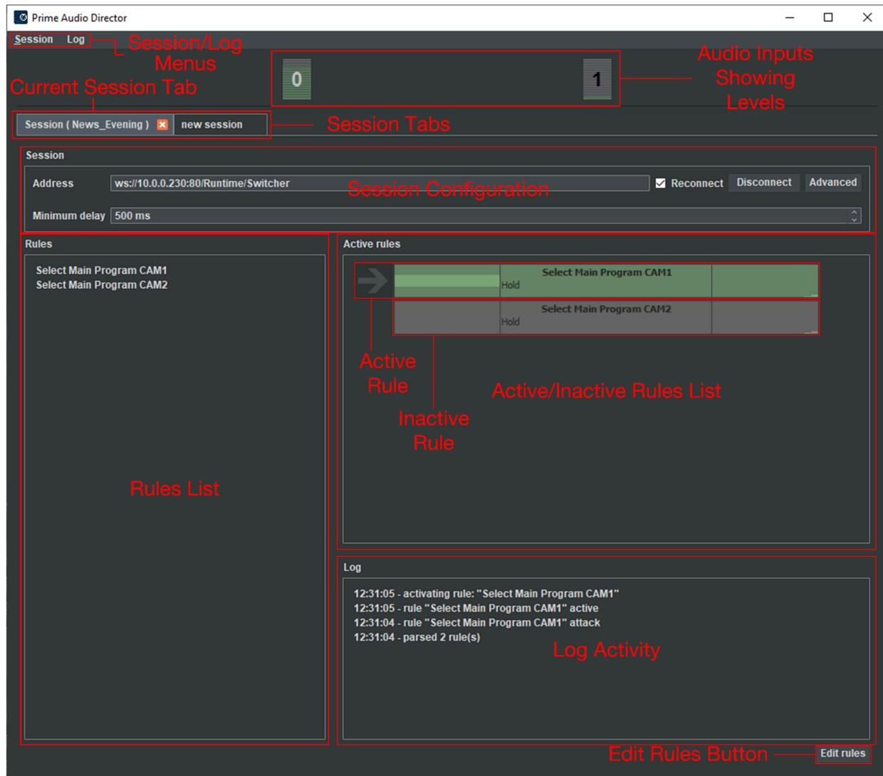
Note that when a session is open, but Audio Director is not connected to PRIME Switcher, the log still displays activity, even though the commands are not reaching PRIME Switcher. This is deliberate, and shows that the rules are operating.
