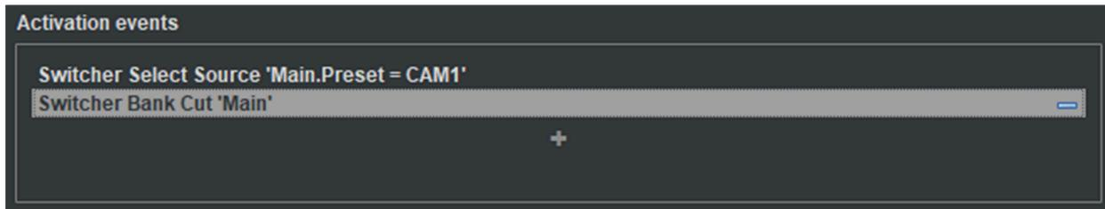
**NOTE:** When planning Activation and Deactivation Events, it is best practice to program the transitions in either the Activation Events or the Deactivation Events - not in both; otherwise, a double transition will be performed. For example:
