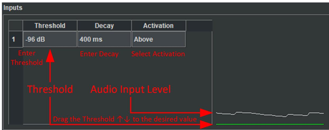
**Activation** specifies at which point the audio input is considered **active**, i.e., **Above** (or at) or **Below** the **Threshold**.
