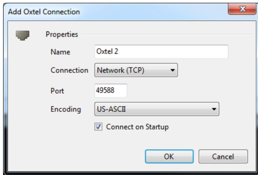
Oxtel commands differ slightly when communicating over serial or TCP. Commands sent over serial port will start with a header (STX0 <02> or STX1 <03>) and end with a two-byte CRC that follow the normal terminator character (a single colon). Furthermore, Oxtel commands received over serial will result in either an ACK or NAK response.
