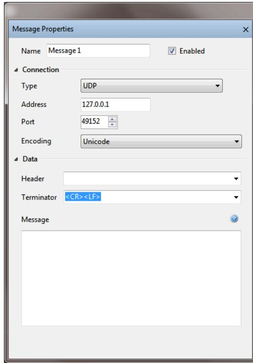
The message property supports common non-printing codes, hex values, and plain text. Codes and hex values need to be surrounded in a tag (angle brackets < and >) to be interpreted correctly. Plain text can be written anywhere and do not require tags. If a tag is not recognizable, it will be left untouched. If necessary, angle brackets can be escaped with a leading backslash (\<).
