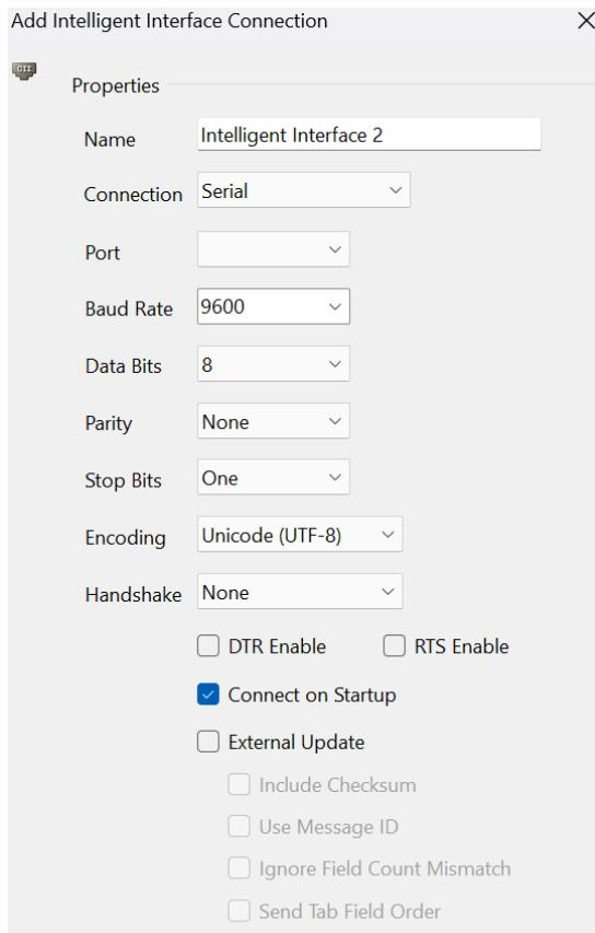
As with the encoding property, there must be parity between the serial port settings configured for the Intelligent Interface connection and the automation system that will be sending commands.
